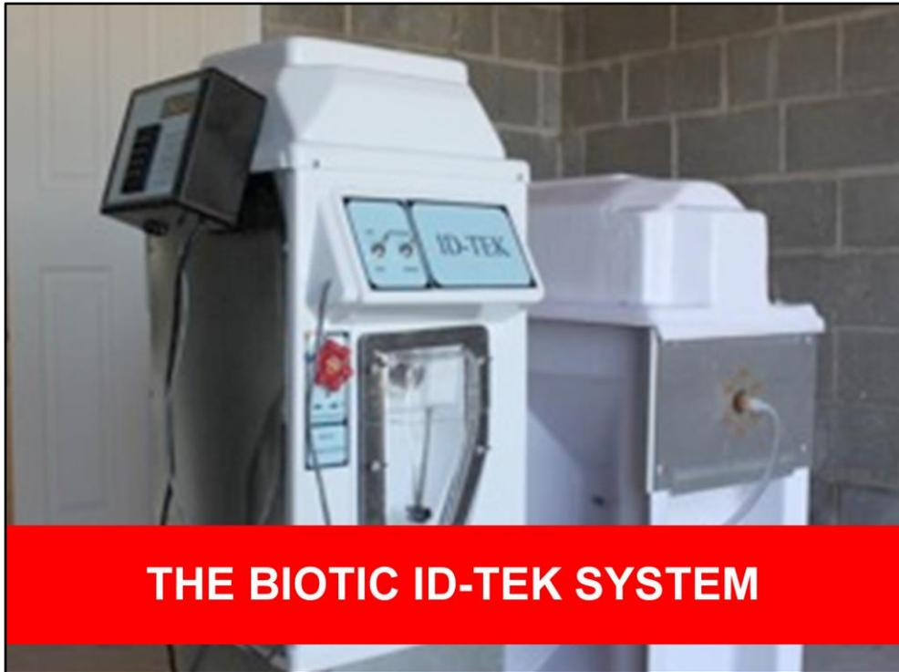
The ID-TEK system takes the automatic feeding system one step further by making it possible to program and control individualized meals for each calf .
